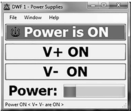
FIGURE 5.7 5 V and –5 V analog discovery power supplied to the inverting amplifier.
