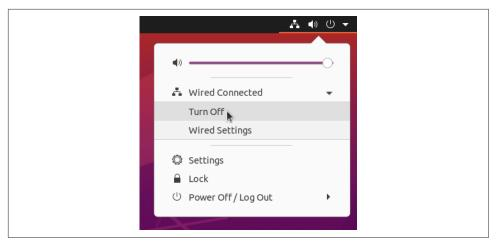
Figure 14-1. Disconnect from the network with NetworkManager
