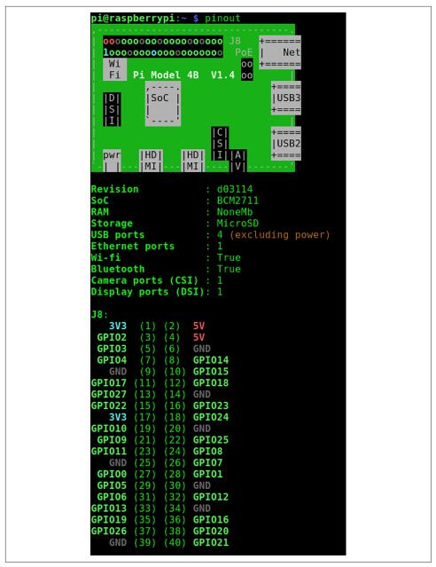
Figure 18-5. Pinout diagram generated by pinout command
