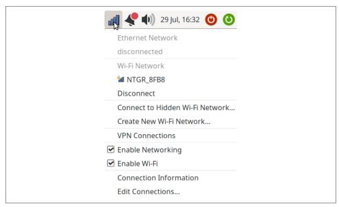
Figure 16-2. Managing network connections with nm-connection-editor
