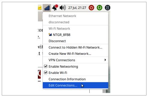
Figure 14-2. Editing network connections in NetworkManager
