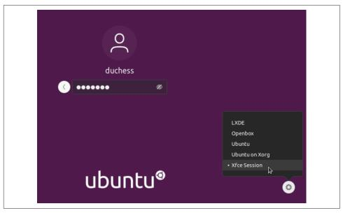
Figure 1-24. Selecting a different graphical environment
