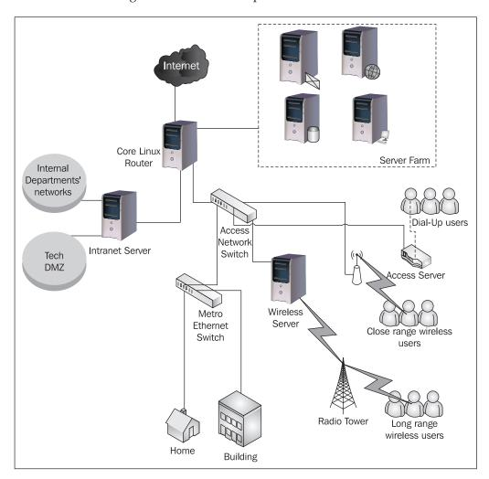
This is a small ISP that has one internet connection, an access network, a server farm, and the internal departments. This ISP uses Linux routers and servers.
