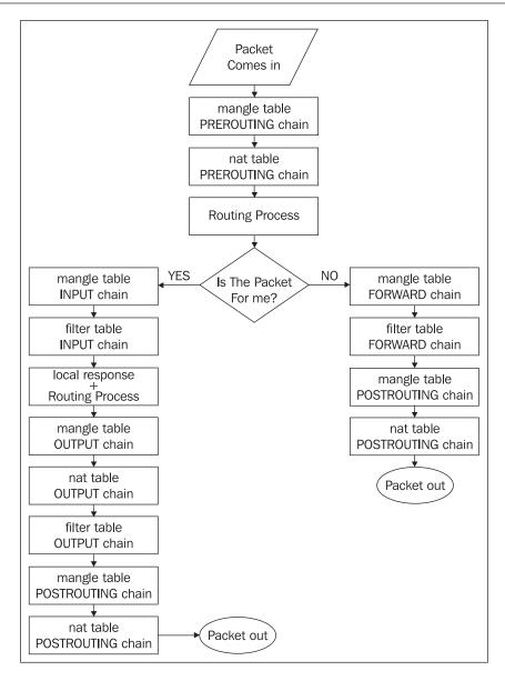
This diagram shows how packets travel the tables and their chains when the NAT and mangle modules are loaded into the kernel. Immediately after a packet arrives at our Linux box, the mangle table PREROUTING chain is analyzed. At this point we can do all sorts of modifications on the IP packets supported by the mangle table (e.g. TOS byte modifications, marking packets, and so on) before the routing process takes place.
