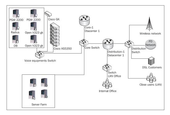
Core-1 has one interface connected to the core switch of Datacenter-1. The voice equipment has special designated racks, and it has its own switch and their own VLAN.
