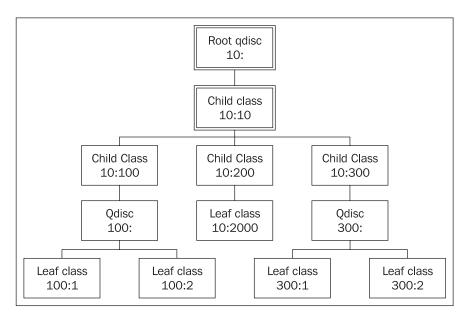
So, basically CBQ or HTB qdiscs allow us to create child CBQ or HTB classes, which we can set up to shape some kind of data. For each child class, we can attach a qdisc for scheduling packets within that child class. Next, we can create leaf classes, which are child classes of the qdiscs we attached to the child classes, or we can create leaf classes as child classes' child classes attached to the root qdisc.
