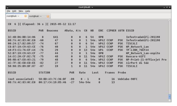
We can distinguish them for the type of encryption used (the fake AP uses Open authentication), the channel and for other fields such as the beacons and data packets transmitted, and the signal power level (Pwr). A lower negative value of the Pwr field means a higher signal level. The signal level of the honeypot AP should be higher than that of the genuine AP, to lure clients to connect to it.
