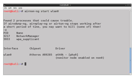
The airmon-ng tool also indicates us the chipset and the driver in use by the adapter. Notice that the mon0 interface is created with monitor mode enabled, while the wlan0 interface is in managed mode (which is the default mode for wireless adapters), as shown in the following output of the iwconfig command:
