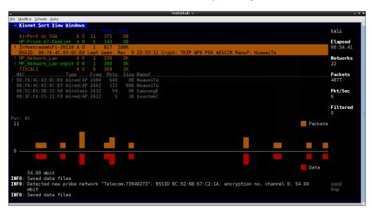
Navigate to **Windows** | **Network Details** for more detailed information, such as the BSSID, the channel, the manufacturer, the signal level, packet rate, and so on:
