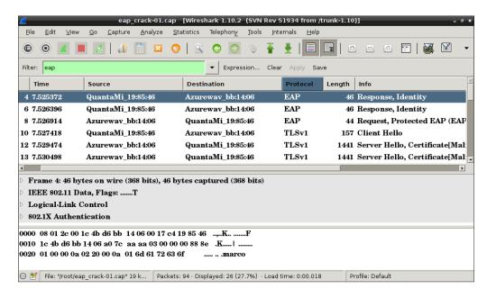
5. Scrolling down the packet listing panel, we will notice the EAP handshake packets in the **Info** column, as shown in the following screenshot:
