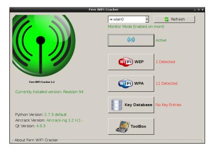
We click on the **Wi-Fi WEP** button, which opens a window showing the detected WEP networks on the top.
