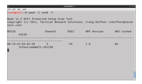
Wash displays information about the detected APs, such as the BSSID, the channel, the WPS version used, whether WPS is locked or not, and the ESSID.
