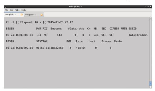
This command saves all the captured frames to the wep\_crack pcap file. We will see how to crack the WEP key when there are clients connected to the AP and when there are no clients.
