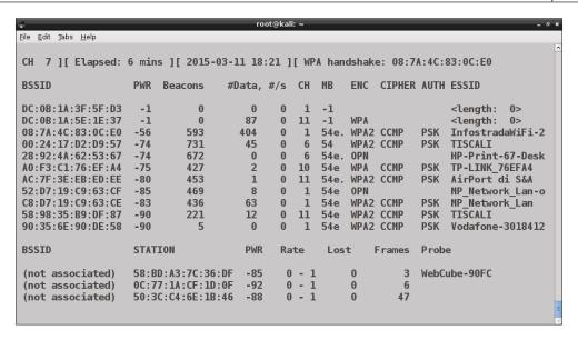
The first line shows the last association between an AP and a client, with the current channel, the elapsed running time, and the security protocol used. As we can notice in the preceding screenshot, the top half of the screen displays the APs while the bottom half displays the clients.
