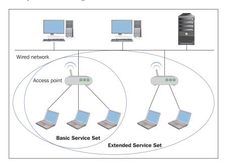
Access points periodically send out broadcast beacon frames to announce their presence. Typically, the beacons also contain the SSID of the AP, so that it is easily identifiable by clients, which can send authentication and association requests to the AP, to connect to the wireless network.
