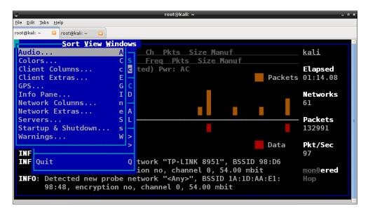
The screen is divided into the following main sections, from the top to the bottom: network list, client list, packet graph, status, and the general info side panel on the right. You can choose which sections to visualize in the **View** menu:
