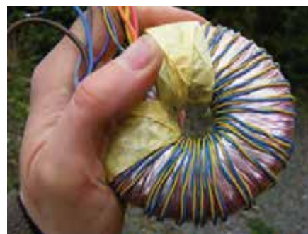
Fig. 15. Occasionally, an extra winding can be added to a toroidal transformer to produce an extra 'free' low-voltage supply. It's a bit labour intensive, but it's got me out of a hole occasionally!
