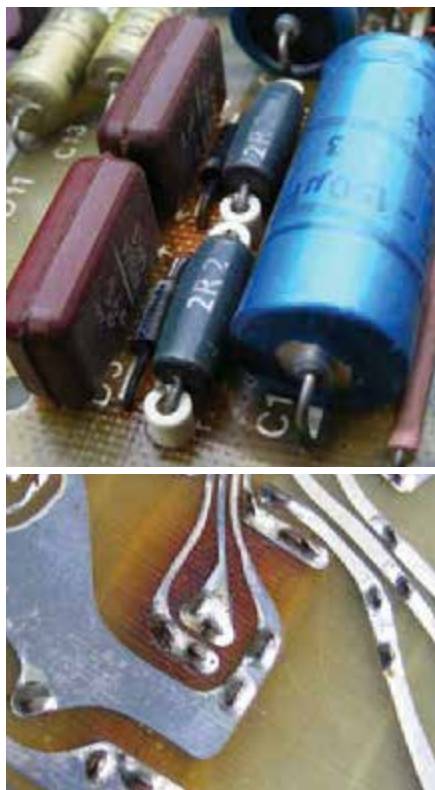
Fig.3. Zener regulators often dissipate a watt or two. Make sure the board doesn't get cooked – put resistors on stand-offs and well away from electrolytic capacitors.
