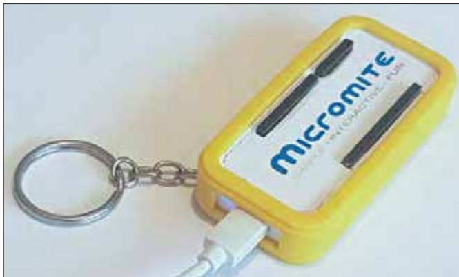
Fig.1. Inside and out – the Micromite Keyring Computer ; built on stripboard with a handful of inexpensive components.
