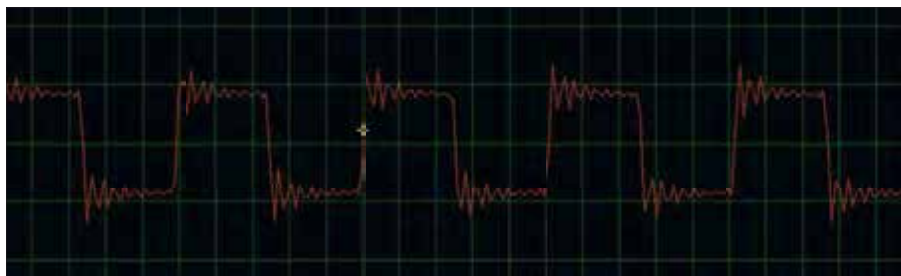
Fig.16. Square wave with low-pass filter resonance.
