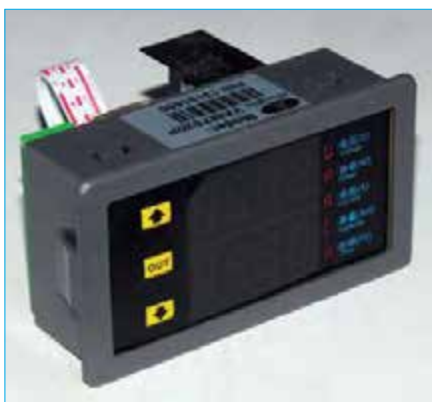
This versatile panel meter can measure and display volts, amps, watts, hours and amp-hours. It can be powered by the supply it is measuring (from 10-75V) and cope with up to 10A current.
