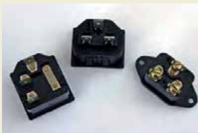
Fig.3.27. Three IEC (male) chassis/panel connectors viewed from the rear. The screw-terminal version (on the right) should be avoided as it is difficult to insulate the screwed connections.
