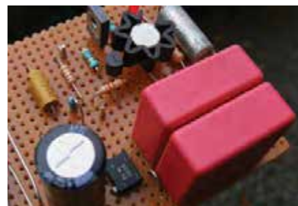
Fig.6. Capacitive droppers are big, but at least they don't get hot – see the circuit in Fig.17.
