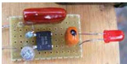
Fig.10. Single-capacitor LED circuit.
