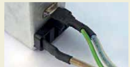
Fig.3.29. Use heat shrink sleeving to insulate connections made to switches, fuses and connectors.
