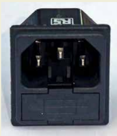
Fig.3.26. An IEC (male) chassis/panel connector with a built-in equipment fuse
