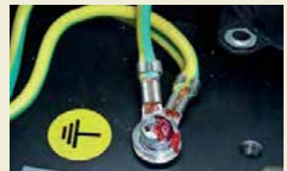
Fig.3.30. A good earth connection should be made to all metal case and chassis parts
