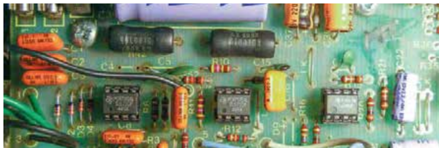
Fig.11. Guitar amplifier – the three TL072 dual op amps are fed from a \pm 30V supply using Zeners. Note the over-rated 680Ω 2W resistors (in black) – a good long-lasting design.
